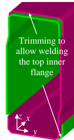
(g) Full Perimeter and Internal (hidden) Flanges (FPIF)
