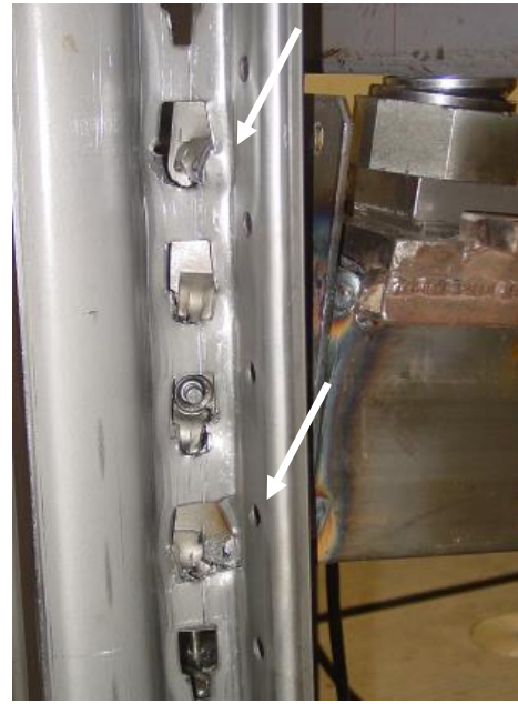
(b) Hooks and perforations tearing (rear view of test FPIF-C-ECCS-I)
