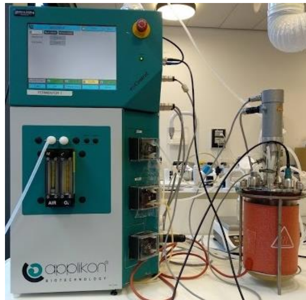
Figure 3.12. Reactor set up for enzymatic hydrolysis of partially defatted finés (PDF).
