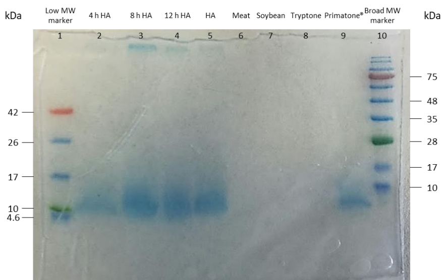
Figure 3.8. SDS-PAGE gel showing the fragments in hydrolyzed samples with Alcalase 2.4L (HA) in the optimal conditions after 4, 8, 12, and 24 h (lanes 2 – 5), meat peptone, soybean peptone, tryptone, and Primatone® RLT (meat tissue) (lanes 6 – 9), Low Range Protein Ladder from 2 to 42 kDa (lane 1) and Wide Range Protein Ladder from 10 to 180 kDa (lane 10).
