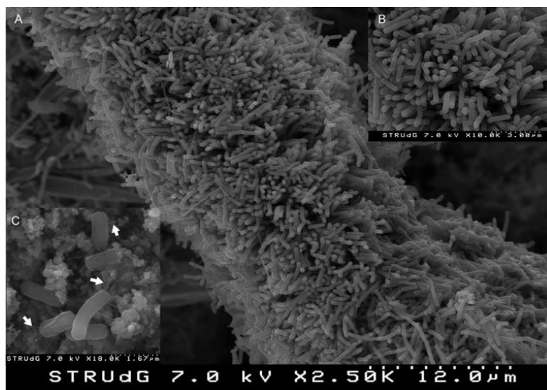
Figure 8. Scanning electron micrograph of the biofilm attached to the cathodes. (A) Colonized carbon cloth fiber. (B) Detail of rod-shaped microbes. (C) Thin appendage-like structures (white arrows) between microorganisms and carbon cloth surface were observed.
