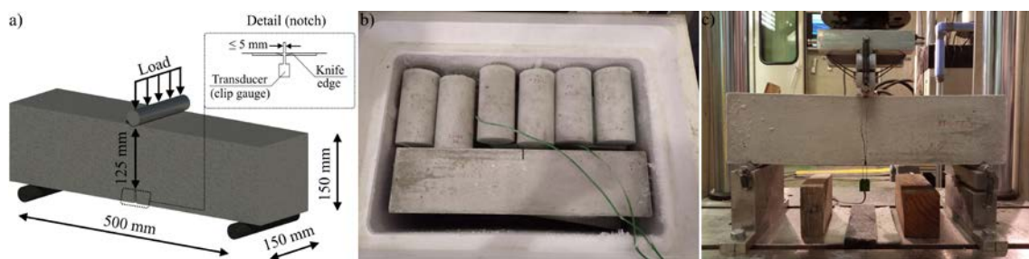
Figure 2 – a) 3PBT at 20°C; b) Freezing procedure and temperature monitoring; c) 3PBT at –30°C
