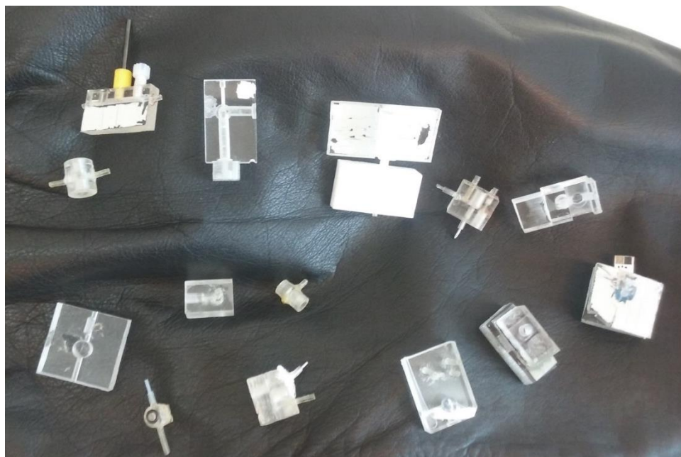
Figure 5.4 An exemplary range of the flow cells fabricated for and tested with glassy carbon and paper electrodes.
