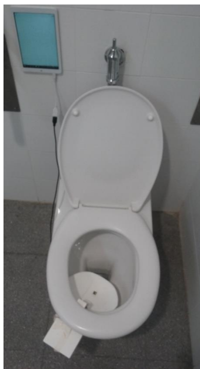
Figure 8.4 The Smart Toilet installed with tablet computer connected and mounted to the wall
