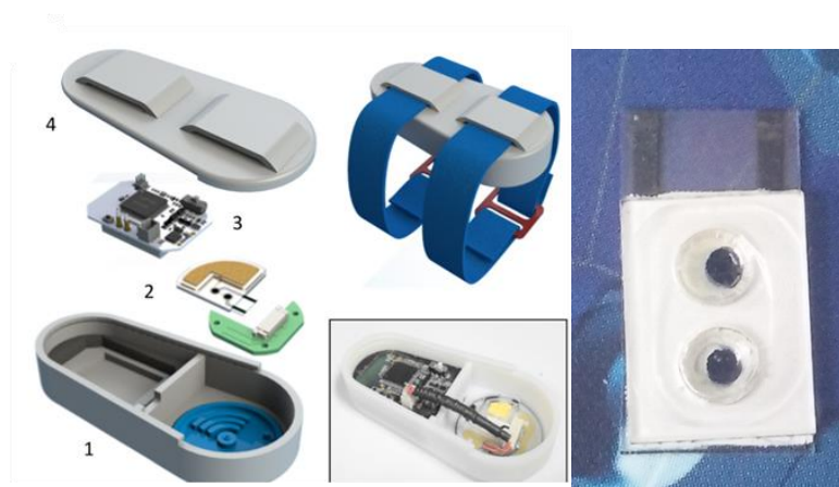
Figure 6.3 Left: The ‘Sweatch’ platform for sodium monitoring in sweat (from [5]) with horizontal arrangement of electronic and fluidic components consisting of 1: sweat harvesting device in 3d-printed platform base; 2: fluidic sensing chip, 3: electronic data logger and battery, and 4: 3D-printed upper casing. Right: one of the screen-printed disposable potentiometric cells used in the Sweatch platform.
