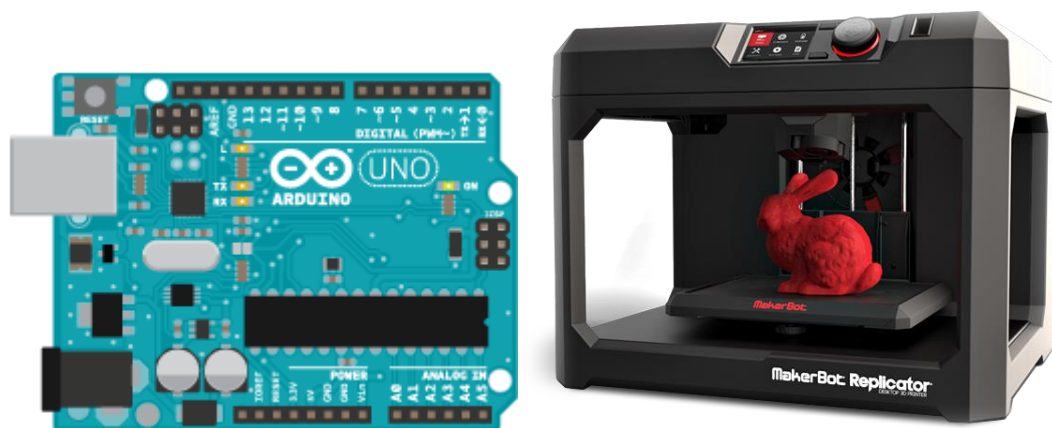
Figure 1.5 Tools of the Maker. Left: An Arduino Uno microcontroller. Right: A 3D printer by Makerbot .
