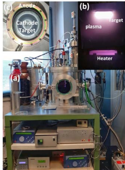
Figure 2.10. Magnetron Sputtering setup used for the growth of RNMO ( R = \text{La}, \text{Pr} ) thin films, located at the ICMAB.
