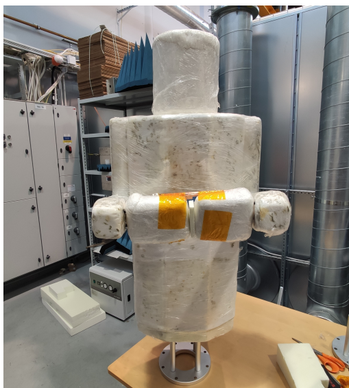
Figure 6.6: Two-hand phantom ready to mount in the anechoic chamber.
