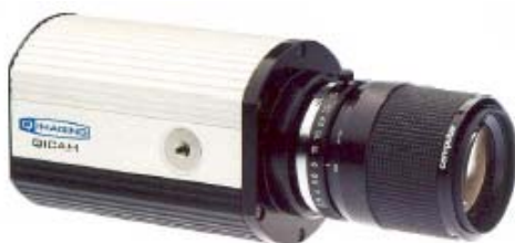
Figure 3.2 Colour CCD camera QImaging QICAM of 10-bit digitalization depth, and an objective lens Cosmimar Television 16mm, 1:14.
