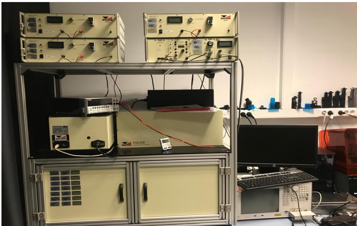
Figure 3.15: Spectral response system used for EQE measurements.
