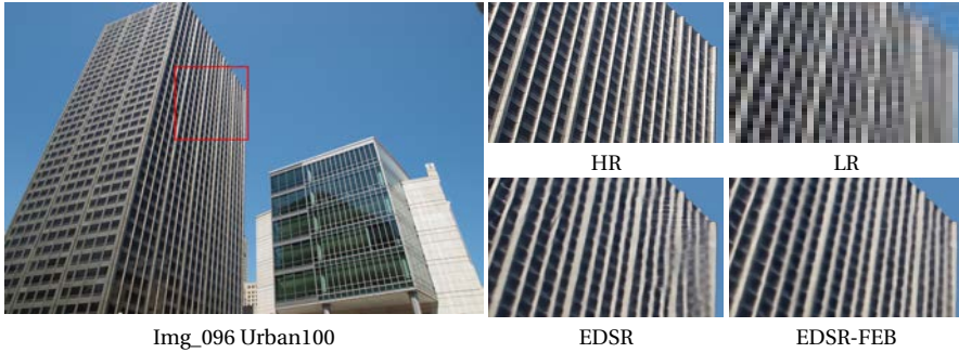
Figure 3.1 – The visual comparison of SR results by the networks with different building modules for scale factor \times 4 . The residual block is used as building module for EDSR. In EDSR-FEB, we replace residual block with proposed FEB.
