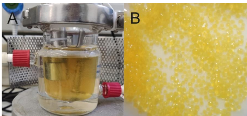
Figure 4.2.2. (A) Customized reactor for use of the NIR probe. (B) The EO-rROL biocatalyst after 10 consecutive reaction cycles as seen under a binocular loupe.
