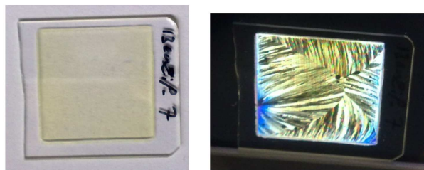
Figure 9.2.: The picture on the left shows one of the studied thin polycrystalline film of benzil under standard illumination. The picture on the right was captured after putting the same sample between crossed polarizers.
