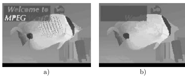
Figure 5.22: Example of size-oriented simplification (size threshold to 50 pixels). a) Simple size simplification, b) Size simplification with propagation strategy
