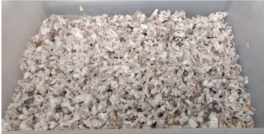
Fig. 3.2. T. versicolor immobilized on Q. ilex wood after 17 days of culture under sterile conditions in a polyvinyl chloride box.
