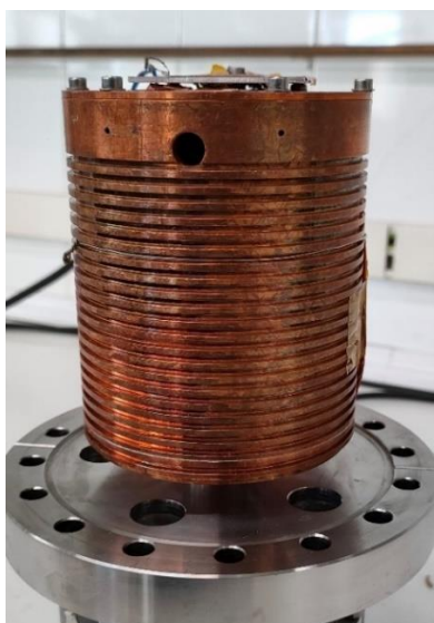
Figure 3. 11. (Upside down) Copper cold trap used to improve the vacuum level in the deposition chamber.
