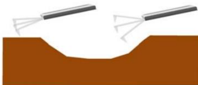
Figure 3. 9. Sketch of the amplitude oscillation changes in tapping mode to probe the samples' surface.
