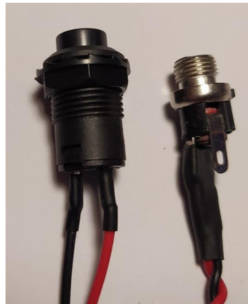
Figure 2. DC-plug socket and pushbutton terminals soldered to their cables.
