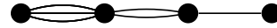
Fig. 6. A multilink Tree T(M) on 4 nodes with set of link-cardinalities M = \{3, 2, 1\} . Its reliability is therefore R_{MT(M)}(p) = (1 - (1-p)^3)(1 - (1-p)^2)(1 - (1-p))
