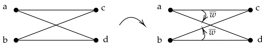
FIGURE 4.2: Rewiring of the edges for a step of the switching algorithm, in the weighted case.
