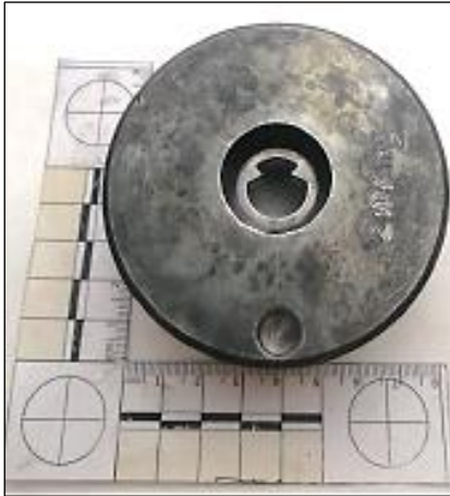
Figure 5.5. Worn hardmetal tool used in catenaries production
