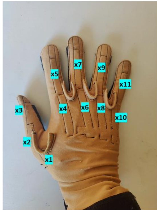
Figure 3.4. Numbering of the sensors used (CyberGlove II®)
