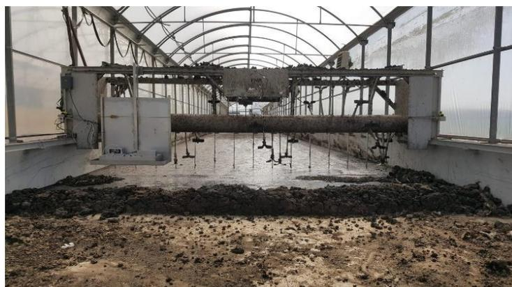
**Figure 26.** Greenhouse solar dryer and turning machine in the semi-industrial installation.
