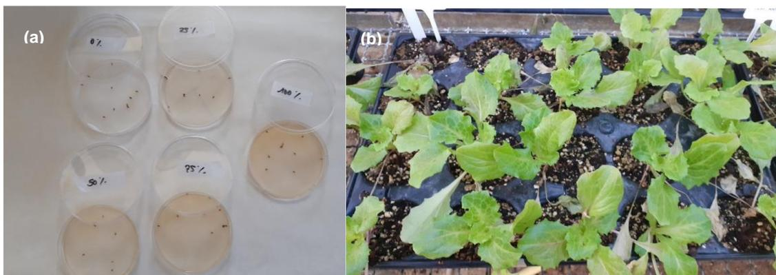
**Figure 15.** Germination (a) and pot trial assays (b) developed in Cabrils to test the phytotoxicity of the produced BBF.
