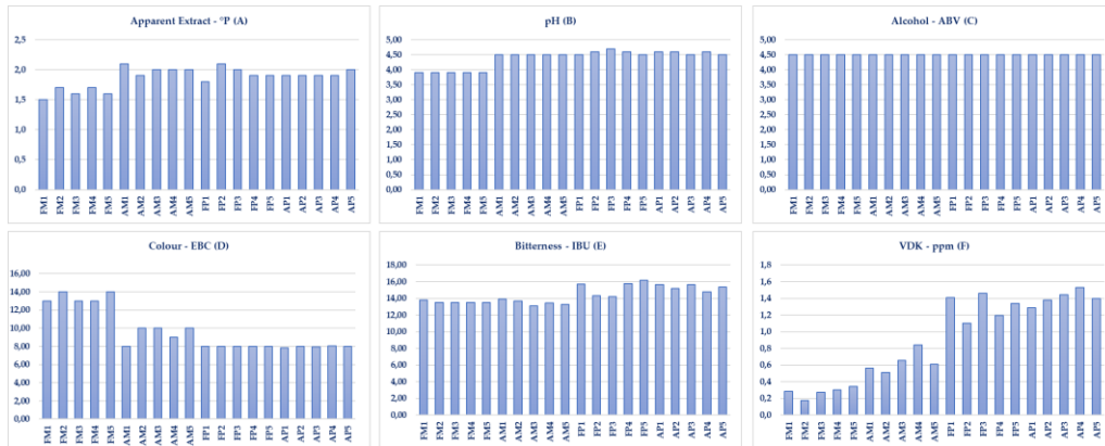
Figure 1. Physicochemical analyses of the beers studied: Apparent Extract °P (A), pH (B), Alcohol ABV (C), Colour EBC (D), IBU (E), VDK ppm (F). FM: Fresh Microfiltered; AM: Aged Microfiltered; FP: Fresh Pasteurized; AP: Aged Pasteurized.
