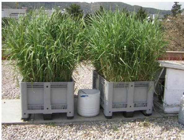
Figure 4.1 Experimental SSF CW fed with municipal wastewater with- or without a physico-chemical pretreatment. The experimental units were located on the terrace of the Marine and Environmental Engineering Building of the UPC.
