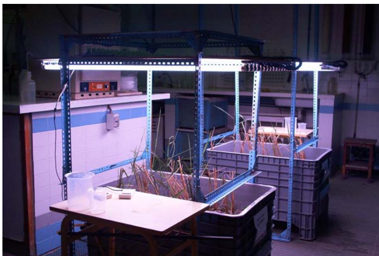
Figure 2.1 Experimental SSF CWs fed with dissolved (glucose) or particulate (starch) organic matter. The experimental units were located in the laboratory of the Sanitary and Environmental Engineering Section of the UPC.
