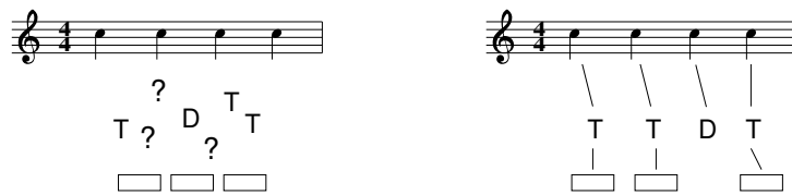
Figure 4.7: A note deletion event in the case of repeated notes with the same pitch forms a problem for mapping, if note positions are not taken into account (left). When note positions are known, the performed notes can be mapped to the nearest score note
