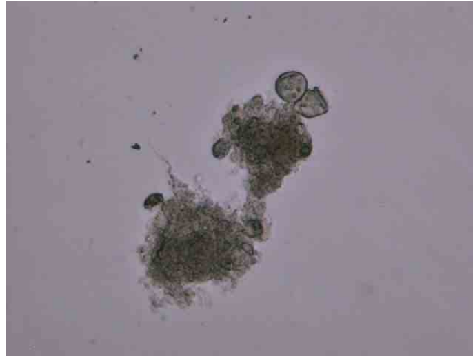
Figure 6-8. Picture of a floc (Magnification: 400X).
