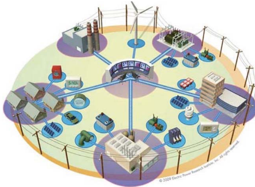
Figure 1.1 Scheme of DGs in the electrical network. Source: Electric Power Research Institute.
