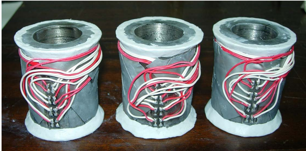
Figure 6.- Load cell for measurement axial loads in bolts.
