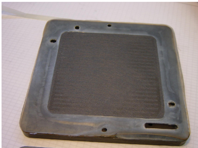
Fig. 12. Cell #5 gasket and diffusion layer which showed no degradation.
