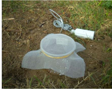
Figure 7. Plastic glass containing ten pupae and soil mixed with perlite. Behind the glass is the data logger which measured the temperature of the subsoil. Photo: E. Peñarrubia.
