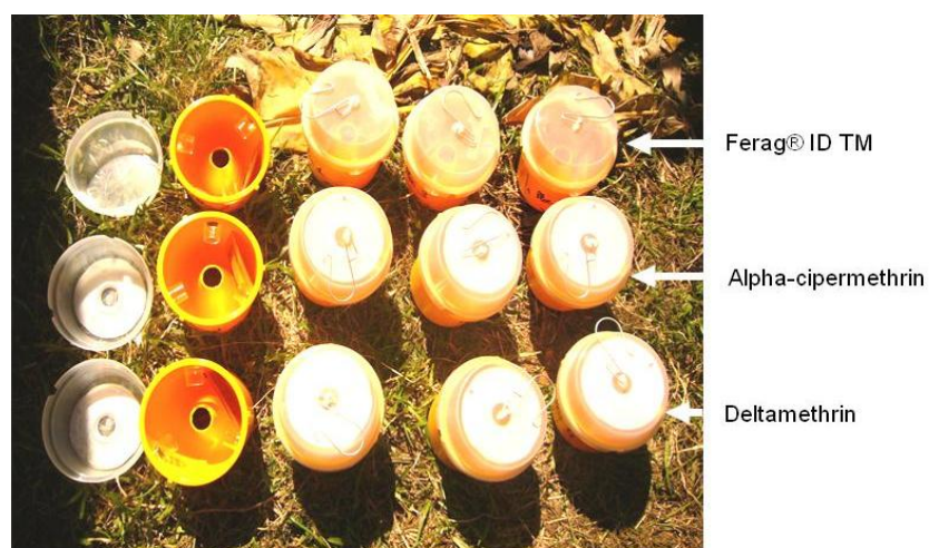
Figure 20. Different insecticides used in the I. trial. DDVP was installed inside the trap and alpha-cipermethrin and deltamethrin in the lid. All treatments were installed in the same model of trap and used the same attractants. Photo: E. Peñarrubia.
