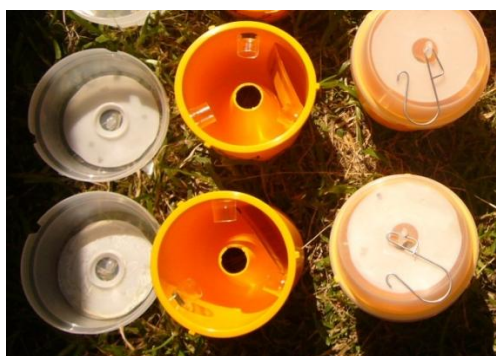
Figure 35. Traps provided with the food lure for medfly and lids provided with the prototype which carries the insecticide tested. Photo: E. Peñarrubia.
