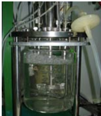
Figures 3.2 Picture of the mechanically stirred bioreactor.
