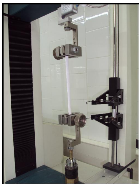
Figure 8. Tensile test setup
