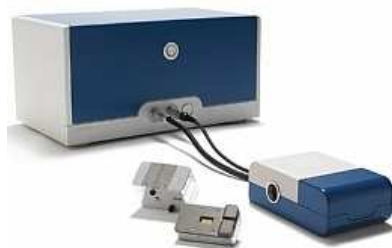
Figure 5.3. QCM-D image. Model E1 from Q-Sense
