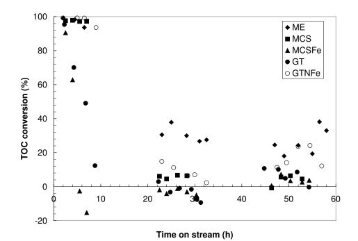
Figure 4.7.4. TOC conversion in TBR reactor using tailored manufactured samples, at 140°C and 2 bar of oxygen partial pressure.
