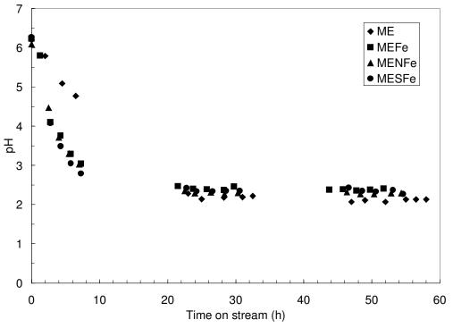
Figure A.5. pH profile of liquid samples from TBR for iron impregnated ACs.
