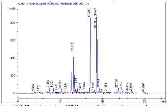
Figure 3.3.2. Chromatogram from HPLC report with intermediate compounds measured at UV wavelength of 254 nm.
