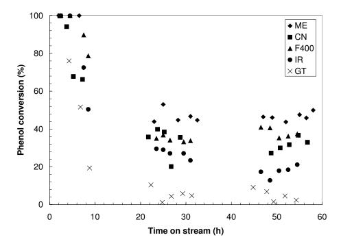
Figure 4.2.2. Phenol conversion in TBR reactor using commercial activated carbons, at 140°C and 2 bar of oxygen partial pressure.
