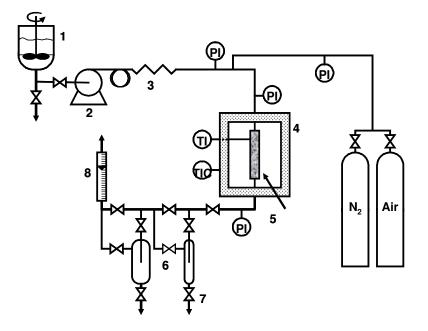
Figure 3.6.1. Experimental Set-up for the CWAO: (1) Feed, (2) High pressure liquid pump, (3) Pulse dampener and liquid flowmeter, (4) Oven, (5) Reactor, (6) Separators, (7) Sampling and (8) Gas flowmeter.
