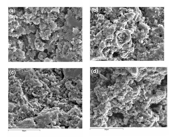
Figure 4.1.2. SEM micrographs of thermally treated samples. (a) ME, (b) ME400, (c) ME700 and (d) ME900.
