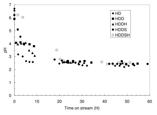
Figure A.1. pH profile of liquid samples from TBR for HD's carbons.
