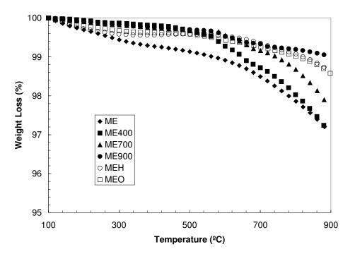
Figure 4.1.6. TGA profiles of the original ME and thermally modified samples.
