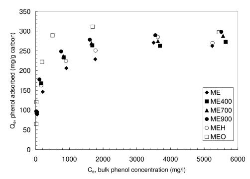
Figure 4.1.10. Phenol adsorption isotherms over activated carbon at 20°C.
