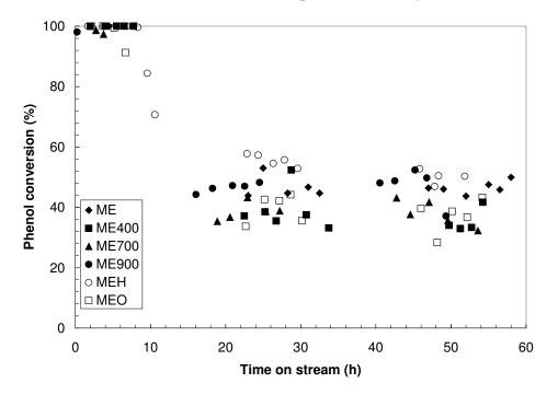
Figure 4.1.11. Phenol conversion in TBR reactor using commercial ME and thermal modified samples, at 140°C and 2 bar of oxygen partial pressure.
