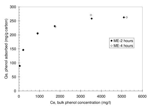
Figure 4.1.9. Phenol adsorption isotherms at 2 and 4 hours.
