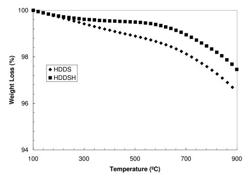
Figure 4.1.16. TGA profiles of the original HDDS and thermally modified sample HDDSH.
