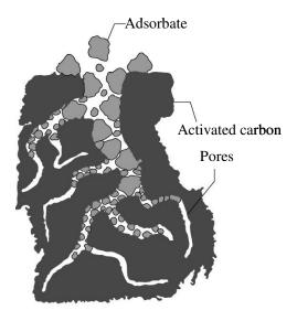
Figure 1.4.1. Internal structure of activated carbon.
