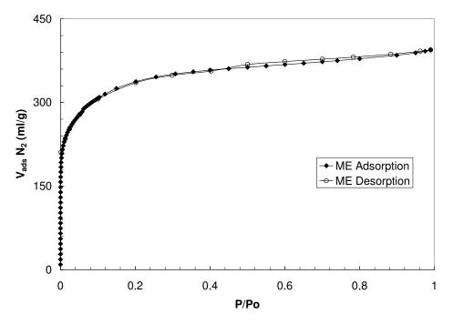
Figure 4.1.1. N<sub>2</sub> adsorption isotherm of carbon ME.
