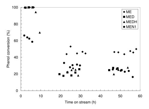
Figure 4.4.2. Phenol conversion in TBR reactor using ME and acid wash modified samples, at 140°C and 2 bar of oxygen partial pressure.
