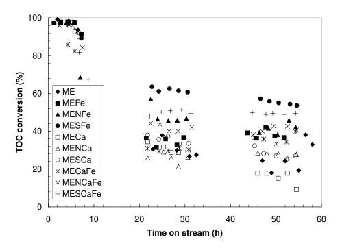
Figure 4.5.6. TOC conversion in TBR reactor using ME and metal impregnated modified samples, at 140°C and 2 bar of oxygen partial pressure.
