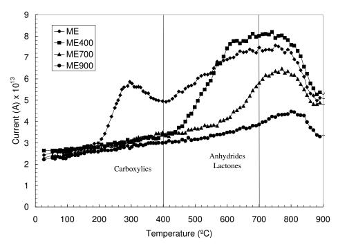
Figure 4.1.3. Signals from mass spectrometer CO<sub>2</sub> released.
