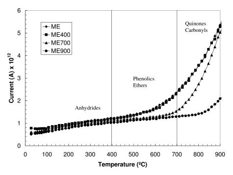
Figure 4.1.4. Signals from mass spectrometer CO released.
