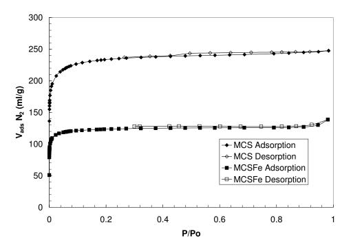
Figure 4.7.1. N<sub>2</sub> adsorption isotherms on tailored carbons.
