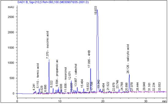
Figure 3.3.1. Chromatogram from HPLC report with intermediate compounds measured at UV wavelength of 210 nm.
