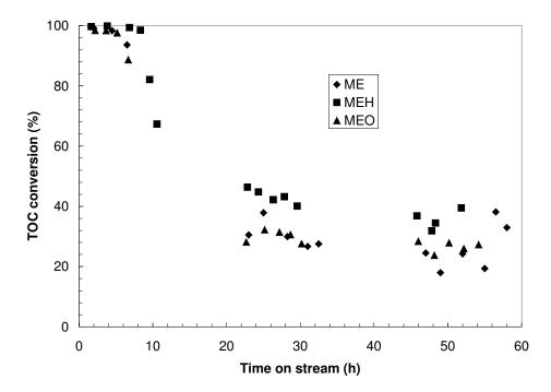
Figure 4.1.13. TOC conversion in TBR reactor using commercial ME and thermal modified samples, at 140°C and 2 bar of oxygen partial pressure.
