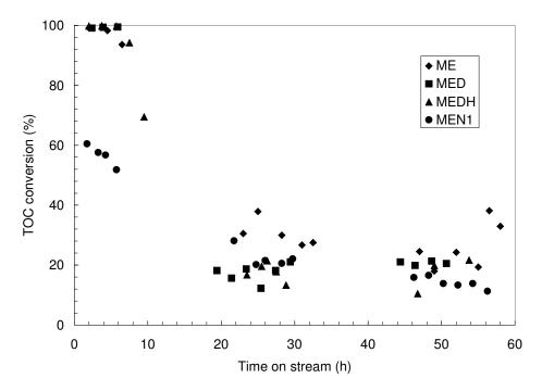
Figure 4.4.3. TOC conversion in TBR reactor using ME and acid wash modified samples, at 140°C and 2 bar of oxygen partial pressure.
