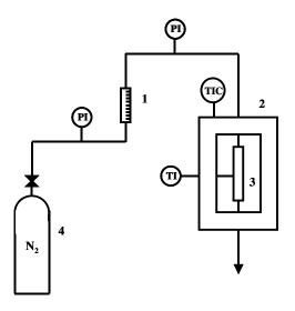
Figure 3.4.1. Experimental set-up for AC modifications: (1) Gas flowmeter, (2) Oven (3) Glass reactor and (4) Gas cylinder.
