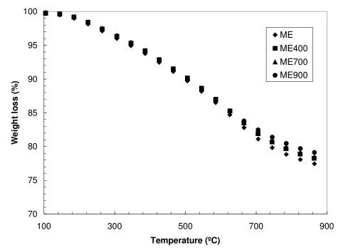
Figure 4.1.14. Weight loss for original and modified ME's after being used as catalyst.
