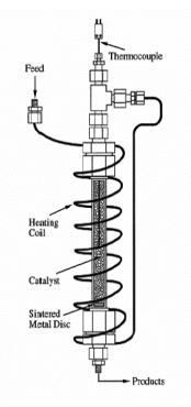
Figure 3.6.2. Detailed scheme of the fixed bed reactor.
