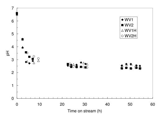
Figure A.2. pH profile of liquid samples from TBR for WV's carbons.
