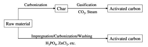
Figure 1.4.4. Basic scheme for the two methods of activation.
