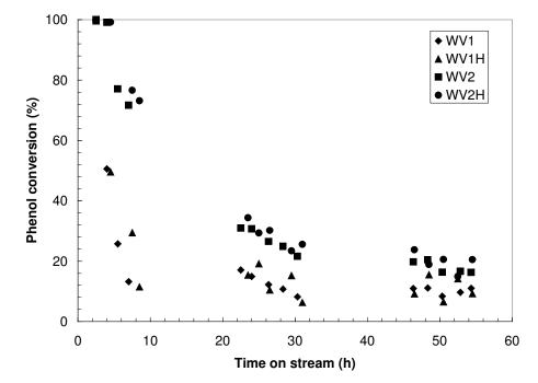
Figure 4.1.23. Phenol conversion in TBR reactor using commercial WV's and thermal modified samples, at 140°C and 2 bar of oxygen partial pressure
