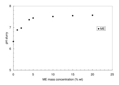
Figure 4.1.8. Mass titration experiment with carbon ME.
