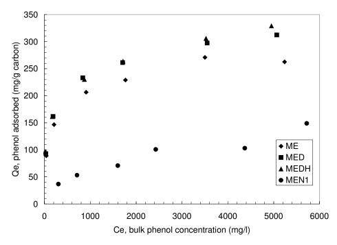
Figure 4.4.1. Phenol adsorption isotherms over activated carbon at 20°C.
