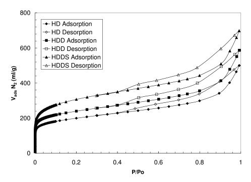
Figure 4.1.15. N<sub>2</sub> adsorption isotherms on carbon HD, demineralised HDD and steam treated HDDS.
