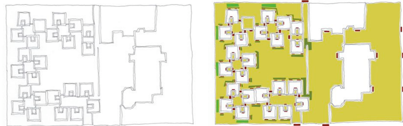
Figure V.89: Hely, Bell and Horne's residential design for Saint John's Village, Glebe, Australia, 1962-1964: access configuration of general set-up (based on original plans and sections as reproduced in D. Mackay, "Viviendas Plurifamiliares: De la Agregación a la Integración", Gustavo Gili, Barcelona 1980, p78-81)
