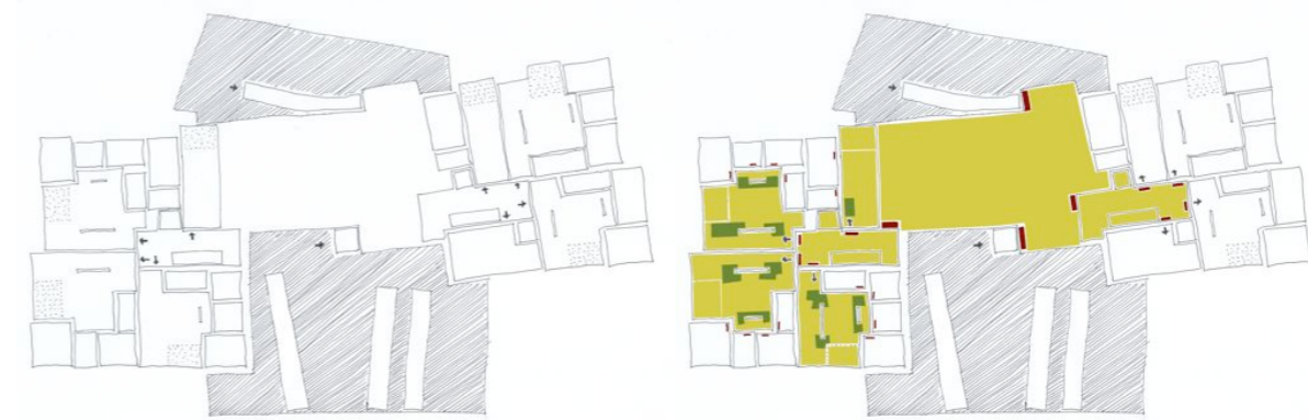
Figure V.15: Alvar Aalto, residential project Hansaviertel, Berlin, Interbau 1957: (left) containing territories and (right) access configuration (based on original plan of the project, ground floor)
