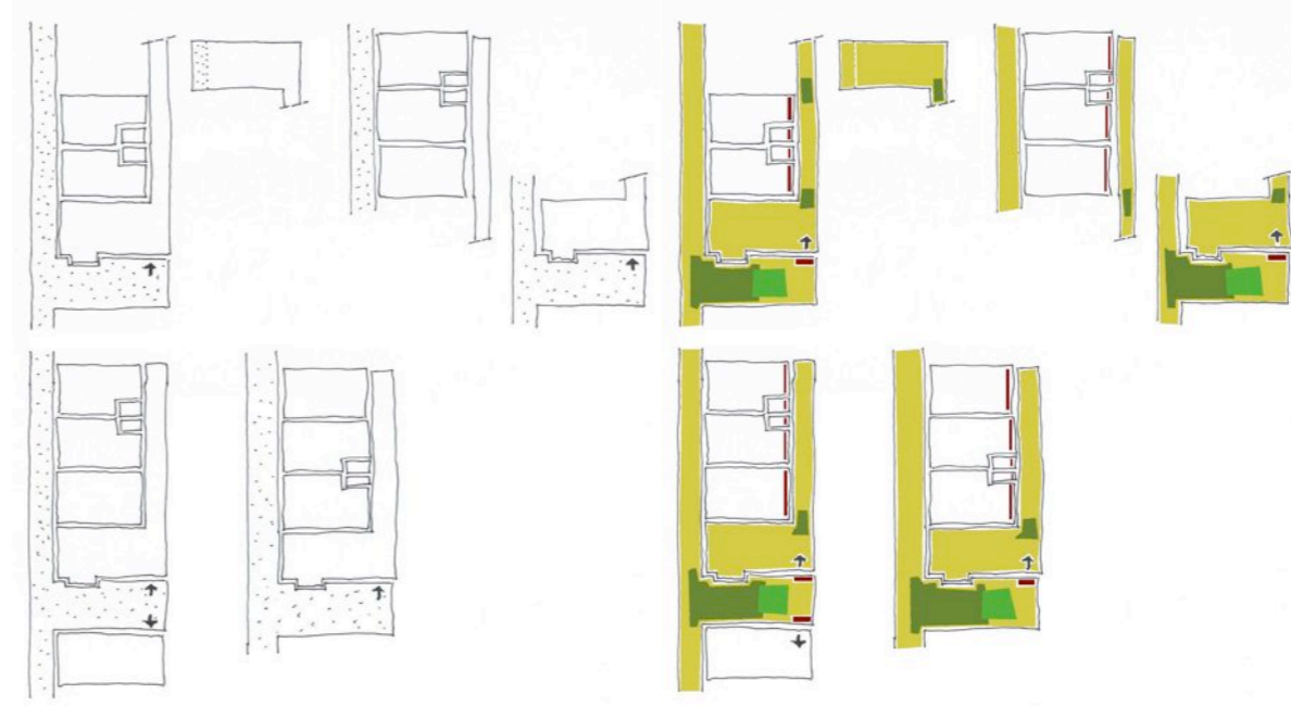
Figure V.21: Kitagata apartments by SANAA, Gifu, (Japan), 1994-2000: access configuration
