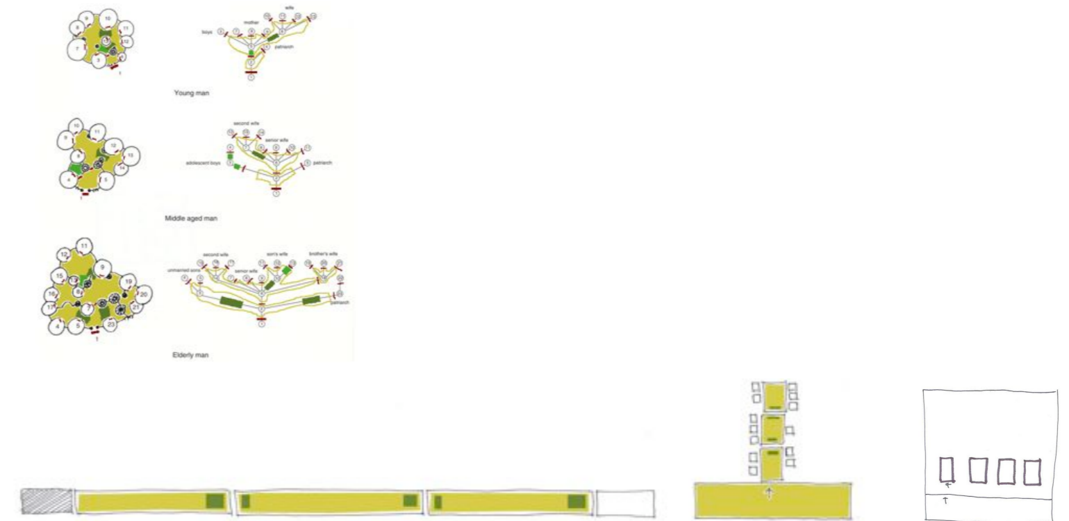
Figure V.14: Tallensi tribe-compound with indication of territorial transition (indication of collective spaces on various degrees: yellow colour), overlap scenarios (indicated in olive green colour), sequential gaps (waiting areas, indicated in green colour) and territorial depth (red strips indicate the change of level of collectiveness within the dwelling)(original fig. 1.4 from J. Hanson, “Decoding Homes and Houses”, Cambridge Univ. Press, Cambridge, 1998, p 15) (right) Tallensi compounds: territorial depth scheme for general lay-out of the settlement
