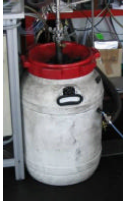
Fig. 3. 37 Barrel were the textile bag to collect CB is placed at the end of the system
