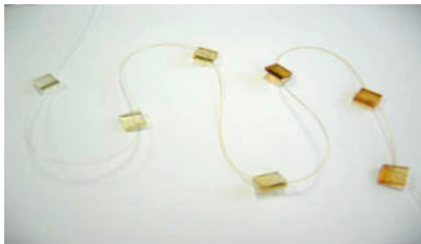
Fig. 3. 17 Glass-pieces used to determine reactive plasma zone in the down-stream reactor
