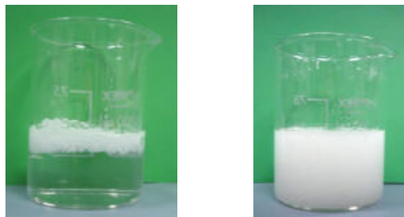
Fig. 3. 22 Polystyrene beads in a water-containing beaker before and after oxygen plasma modification Left and right respectively
