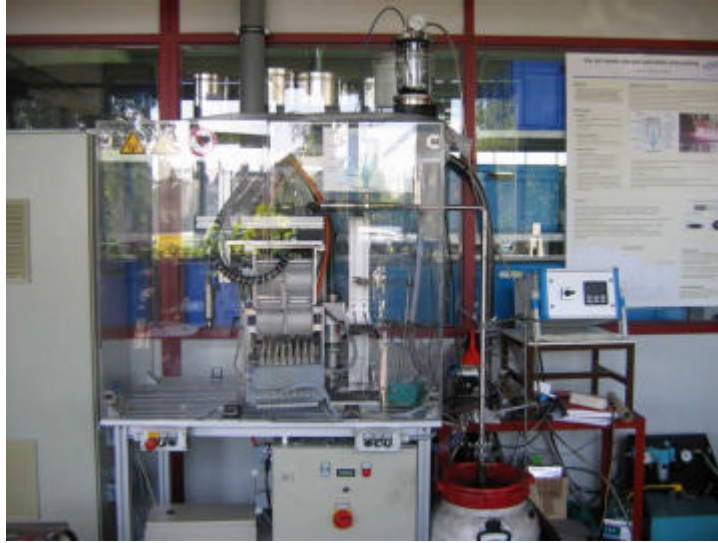
Fig. 3. 39 Picture of the final APP system for powder modification 1:CB container, 2: plasma reactor, 3: cooling pipe, 4: collection system
