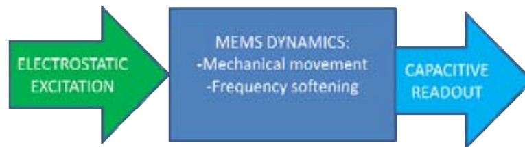
Figure 2.1 Conceptual map which illustrate the working principle of the electrostatic excited and capacitively sensed micromechanical resonator.
