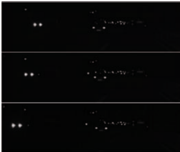
Figure 4.2: Successive frames from a night driving video sequence recorded by an on-board camera. One blob may correspond to two far away light sources or reflections. Blobs merge, split and get occluded by other vehicles, trees and fences.
