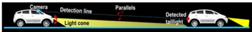
Figure 3.2: Headlight beam control system. The desired light cone is directed parallel to de detection line between the mounted camera and the closest detected vehicle light.
