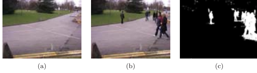
Figure 4.3: (a) Background image, (b) Current frame, (c) Binary moving pixel mask.
